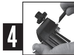
**4** Attach the boom to the cup bracket. Locate the arrow on the inside of the cup bracket base. Insert the boom end in the direction of the arrow all the way through the base of the vane mount. Grasp the silver bungee end AND the transparent bungee washer, then pull the boom back, stretching the bungee. Drop the bungee into the slot and slip the boom end into the opening near the compass. Gently rotate the boom until the angled end "seats" into the base of the opening.
