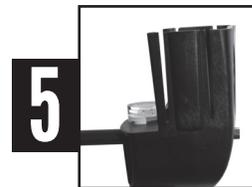
**5** Attach the Vane Mount to your tripod and level your tripod. Spin the Vane Mount knob onto the 1/4-20 mount on your tripod. Slip your Kestrel into the Vane Mount with the display facing the bubble level. Adjust the flight so it is vertical. Observing the level on the Vane Mount, carefully adjust your tripod so the Vane Mount is level and rotates freely and evenly.
