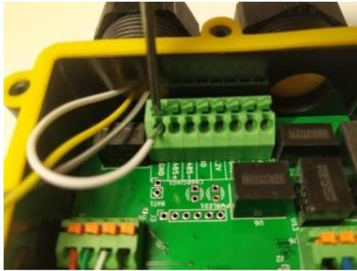
4. Tighten the holder in order to fix the cable and close the gateway with the screws.
